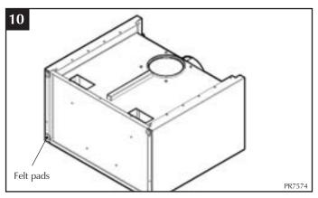
10. Firstly remove all internal parts from the stove and remove the door. Tip the stove onto its front on a soft surface that will not damage the paintwork. Apply felt pads to each corner of the base.
